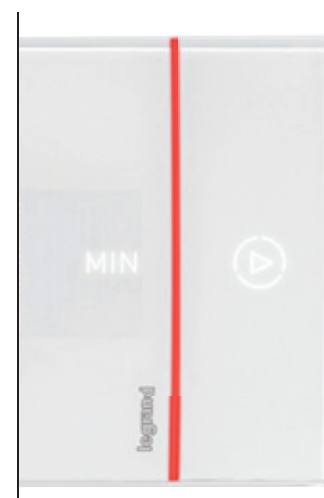
The red bar * indicates that the "Boost" function is active. You can cancel it at any time by clicking on the icon.
