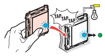
The LEDs of the 2 products flash blue and then light up in solid blue. The wireless control indicator goes off and the connected switch indicator turns green.
